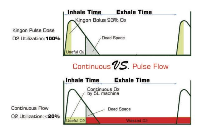
Pulse Dose is based on breathing and inhaling, which is more sophisticated. Pulse Dose mechanisms are more sensitive, utilizing an oxygen conserver and other technology to deliver oxygen based on breathing rates and other factors.
